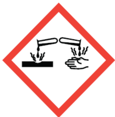
Burns skin Damages eyes Corrosive to metals
