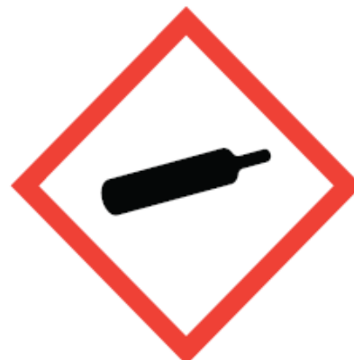
Gas under pressure
